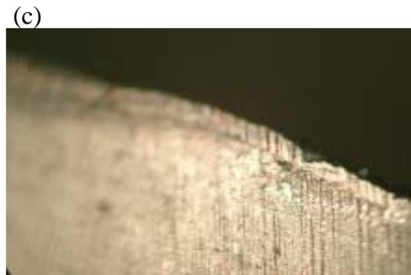
Fig.5-7 Result of high-speed milling test: (a) changes in flank wear and optical images of boundary wear (b) (Ti,Al)N after 50m and (c) (Ti,Cr,Al)N after 70m.
