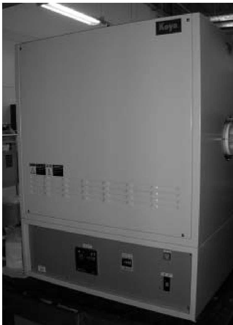
Figure 2.6: Resistive furnace employed in this work.
