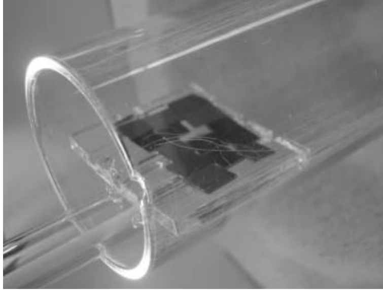
Figure 2.5: Picture of a quartz sample boat equipped with a port for inserting a thermocouple. The boat, on which samples cut into 5 \times 5 \text{ mm}^2 are put, is being inserted into the quartz tube.
