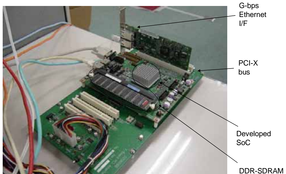
Figure 4-17 Photo of routing evaluation system
