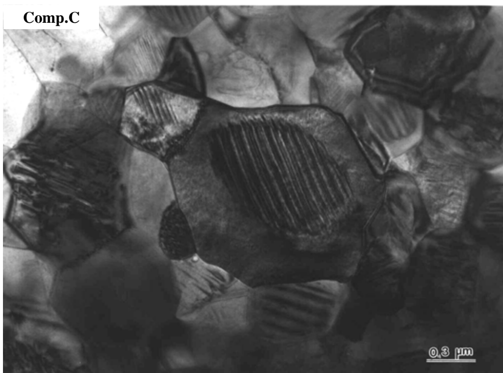
Fig.3-11 TEM bright field images for Comps.N and C fired at 1320°C for 1h.
