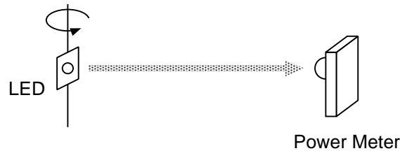
Figure 3.2: Measuring method of radiation pattern.
