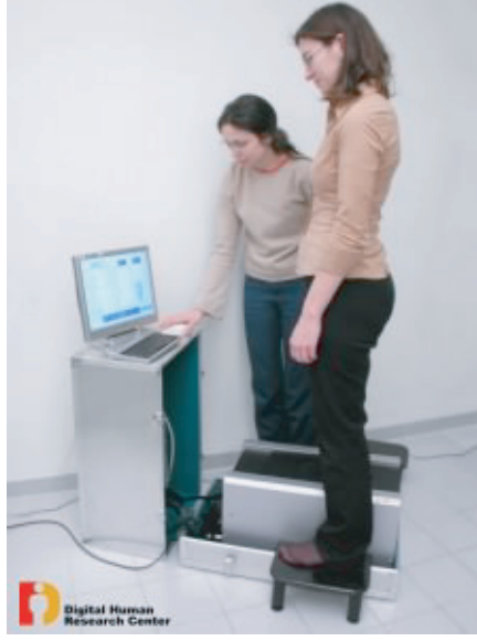
Figure 3.21: The foot models in database are established by measuring the surface position information with a foot scanner[35].
