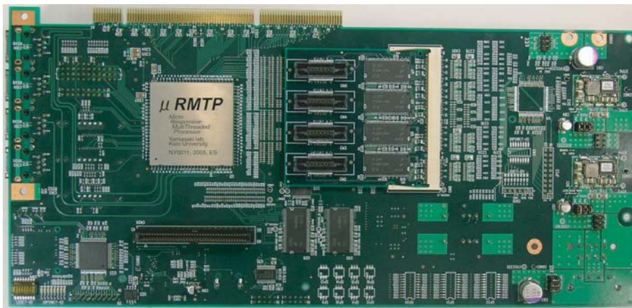
図 6.14: Responsive Multithreaded Processor
