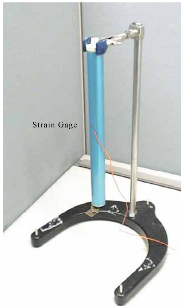
Fig.2.11 Measurement of Twisting Vibration of the Photoreceptor
