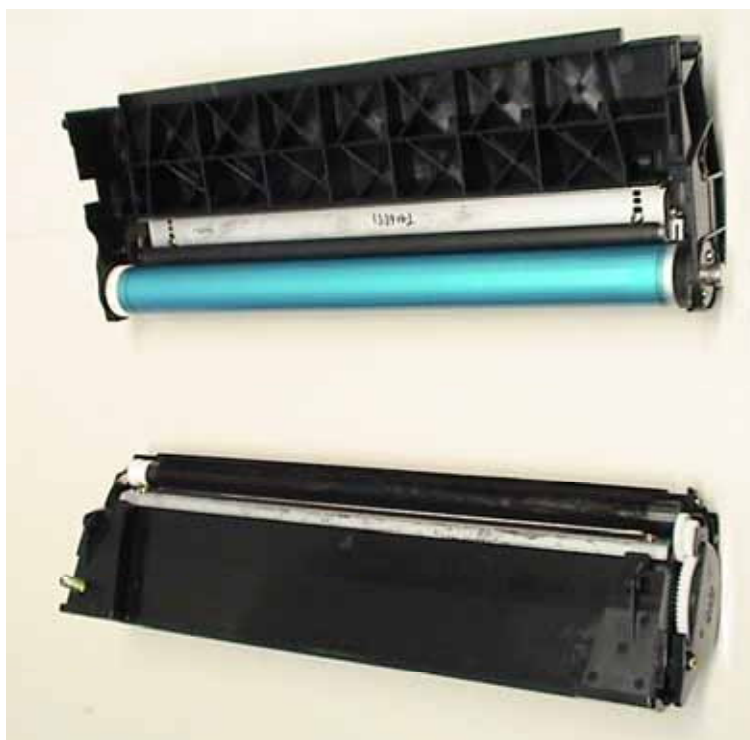
Fig.2.15 Separation of Cleaning Blade and Photoreceptor from Process Cartridge Unit
