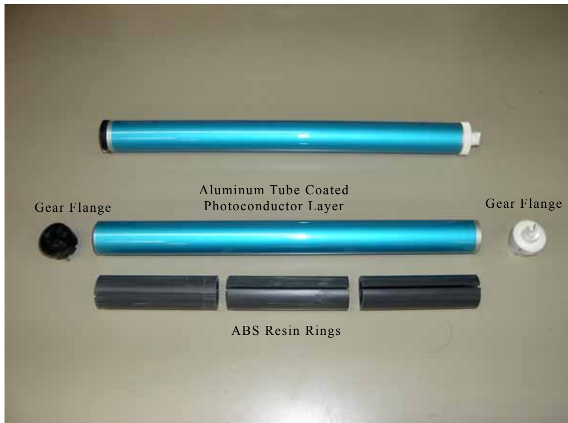
Fig.2.10 Composition of Photoreceptor Assembly Unit
