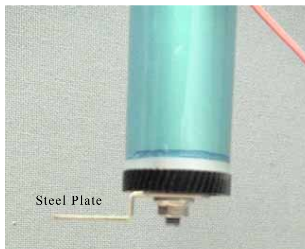
Fig.2.12 Detail of Impulsive Excitation Method
