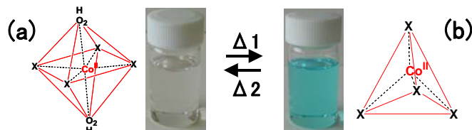
Figure 5-3. Color change of \text{Co}^{2+} ion containing in reverse micelle, toluene / DDAB / \text{H}_2\text{O} , at W = 5 , before and after thermal treatment, (a) before treatment and (b) after thermal treatment at 50\text{ }^\circ\text{C} .
