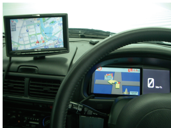
Figure 5. 2 Position of route guidance information of SD providing method (map-type information on the top of the center console, arrow-type information at the place of the dashboard)
