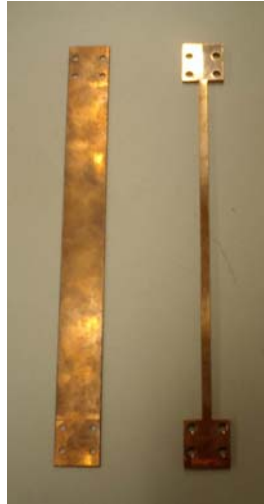
Figure 5.2 Healthy and Damage Columns
