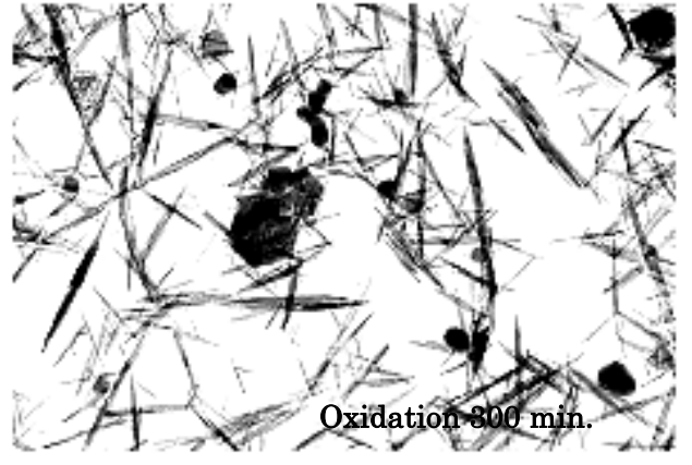
Fig.6-7 TEM figure of the synthesis process goethite particles from \text{Fe}(\text{OH})_2
