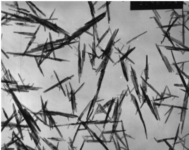
Fig.9-2-1 TEM photographs of goethite particle from \text{Fe}(\text{OH})_2
