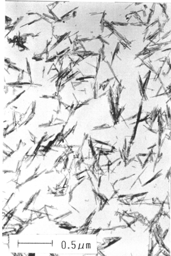
Fig. 3-1(b) Transmitted electron micrograph of acicular goethite (sample X)
