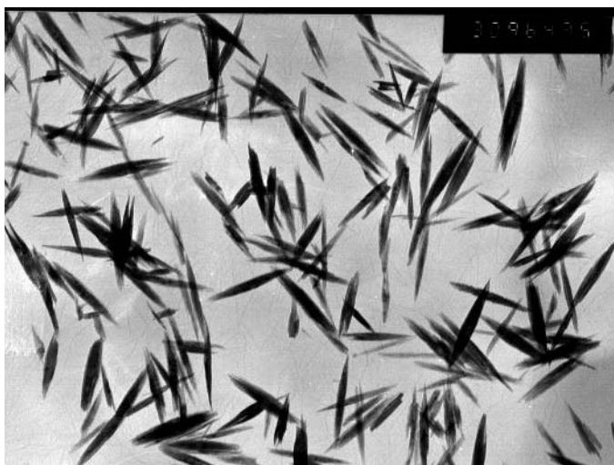
Fig.9-4-1 TEM photographs of goethite particle from \text{FeCO}_3\text{-Fe}(\text{OH})_2
