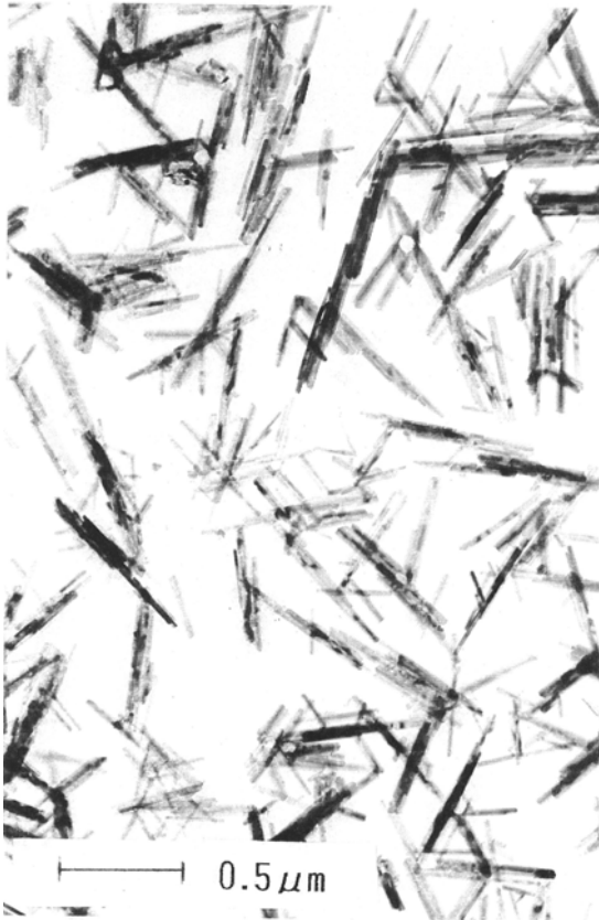
Fig. 3-1(a) Transmitted electron micrograph of acicular goethite (sample XIII)
