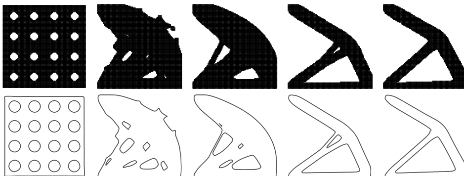
Figure 7.19: Level set (bottom) and \Omega_{matnb} domain (top) time history for 101 \times 101 grid
