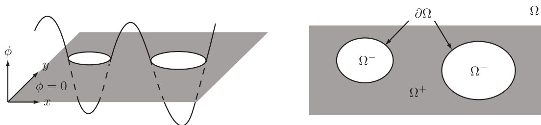
(a) Higher dimensional implicit function (b) Boundaries, lack of and presence of voids in \Omega
