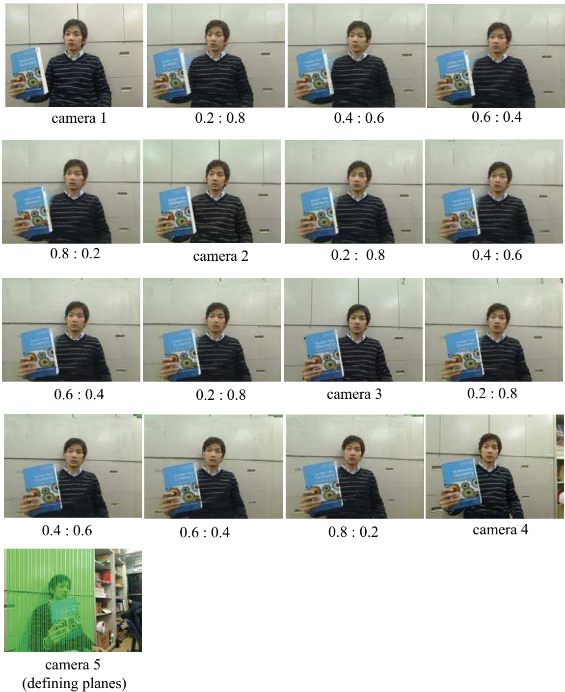
Figure 5.10: New views produced by our proposed plane-sweep algorithm in projective grid space using 80 planes.
