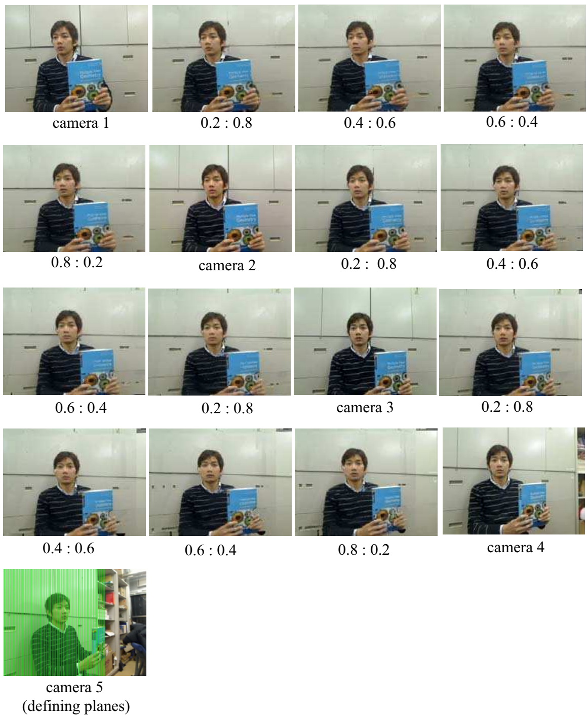
Figure 5.8: New views produced by our proposed plane-sweep algorithm in projective grid space using 80 planes.
