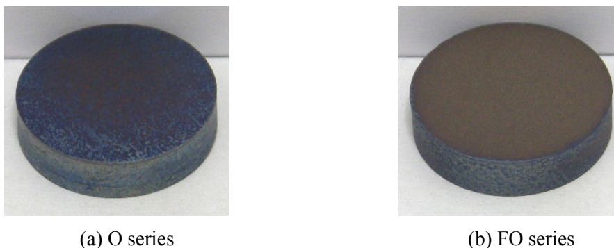
Fig.3-4 Features of oxidized specimen (Treated material: Pure iron, Peening pressure: 0.6MPa, Peening time: 30s, Oxidation temperature: 300°C)
