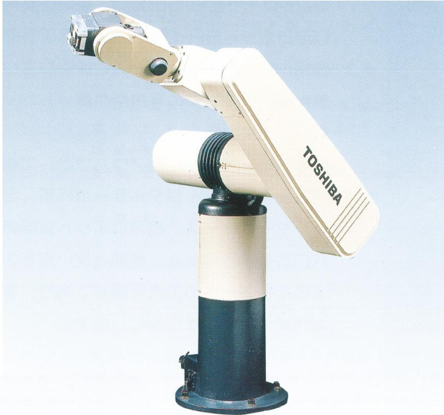
Fig. 1.3 PUMA-type robot arm SR-606V by Toshiba Corporation [16].
