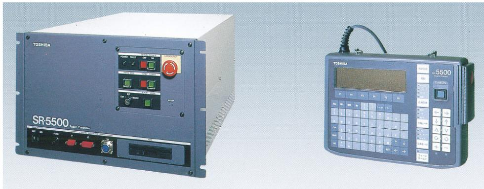
Fig. 3.7 SCARA-type robot arm controller SR-5500 by Toshiba Corporation [16].
