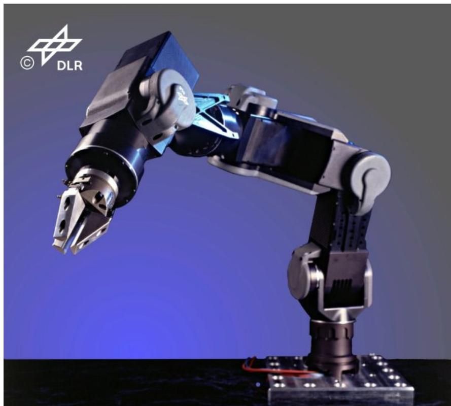
Fig. 2.1 Light-weight robot Version II “LWR II” by DLR [148].
