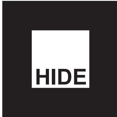
Figure 2.1: Marker for ARToolKit [42]. The main characteristic of ARToolKit is the flexible design of the markers. Inside the black frame, any kinds of asymmetric pattern can be inserted.
