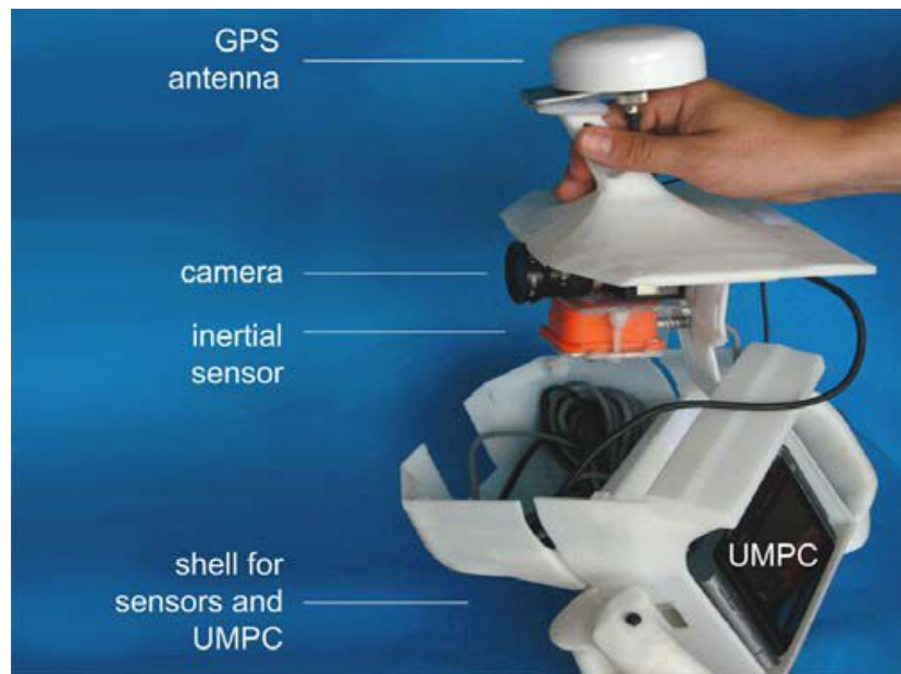
Figure 2.6: Outdoor AR platform. Several sensors are fused to estimate a global camera pose. The augmentation result is displayed on the UMPC. Courtesy of Gerhard Schall [89].
