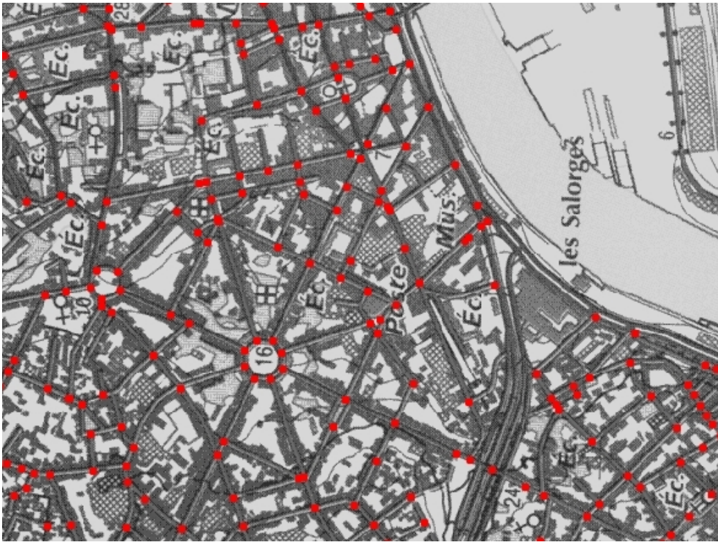
Figure 6.3: Map with red intersections. The map is generated from GIS by using a SQL query to extract intersections from a road network.
