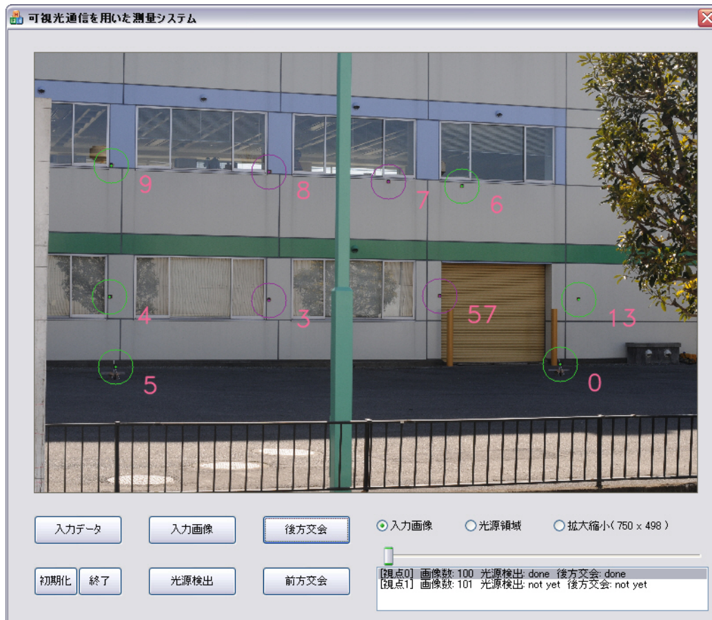
Figure 7.2: GUI. First, a user stores captured images in the camera, and then input them into the system. The user operates the extraction of lights, camera calibration and triangulation on GUI.
