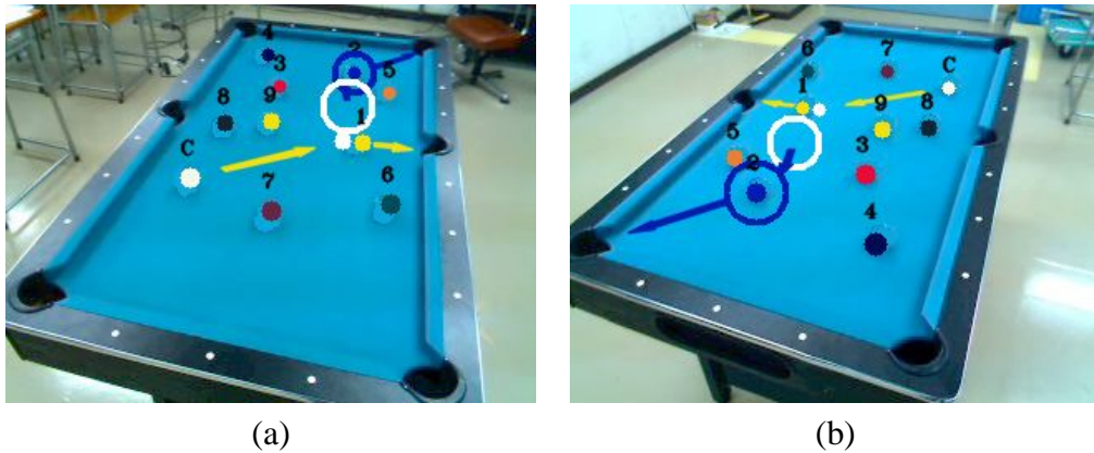
Figure 4.9: Online AR display. (b) is captured from the opposite side of (a). In order to achieve AR for arbitrary views, a camera pose with respect to the table is appropriately computed. In this case, two short sides are identified.
