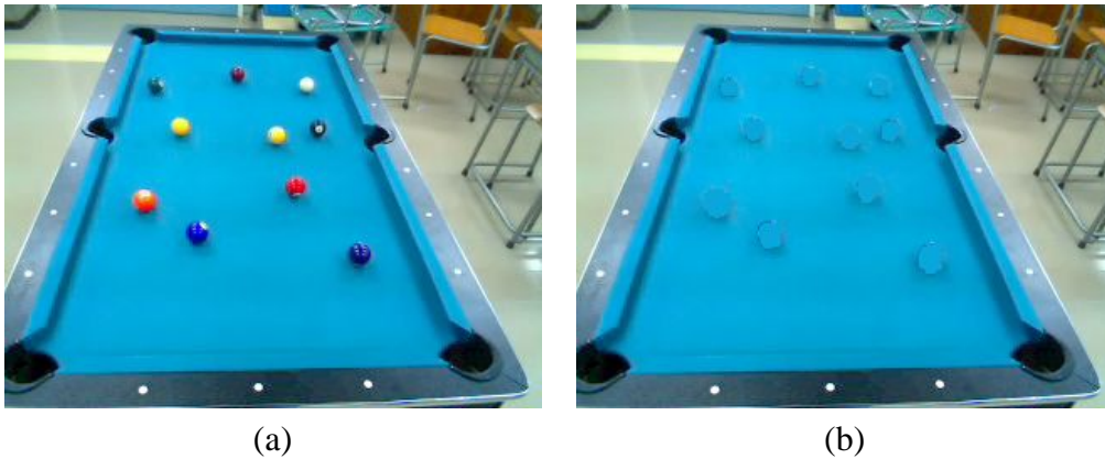
Figure 4.10: Background generation. (a) For a captured image, ball regions are extracted. (b) The ball regions are interpolated by green mat color.
