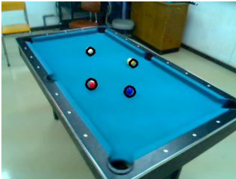
Figure 4.12: Reprojection error. For each ball, the center of a computed ball position in the world coordinate system is reprojected onto the captured image. The distance between the center in the image and the reprojected center is evaluated.
