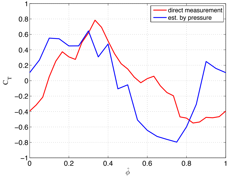
Figure 7.2: Comparison of torque coefficients estimated (“est”) by pressure and torque directly measured by strain gauges for flapping rigid plate at Re=3160 .
