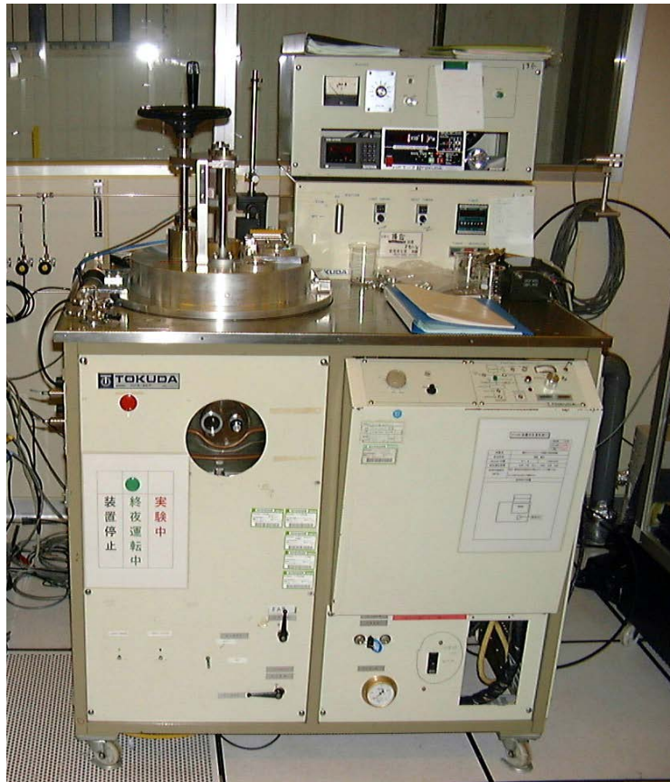
Fig. 2-5 Exterior view of the vacuum chamber
