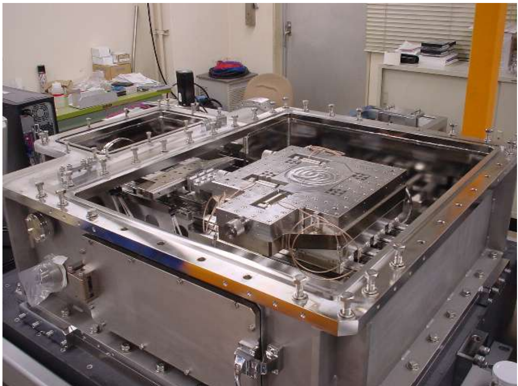
Fig. 3-15 Fine X-Y stage on Coarse X-Y stage in process chamber
