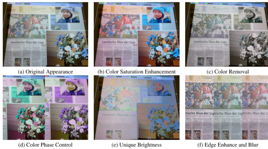
Figure 4.3: Example of appearance control results. (a) Original appearance. (b) Color saturation enhancement. (c) Color removal. (d) Color phase control. (e) Unique brightness. (f) Edge enhance and blur. Courtesy of [Amano and Kato, 2010].
