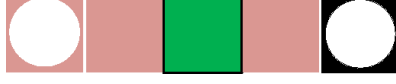
Figure 1.9: NOT gate in MBQC. The input qubit and all pink qubits are measured in the \sigma_x -eigenbasis and the framed-green qubit is measured in an adaptive basis depending on the measurement outcome of qubit 2. A rotation measurement operator on xy -plane around z -axis with angle \pi on qubit 3 makes the qubit 3 not adaptive.
