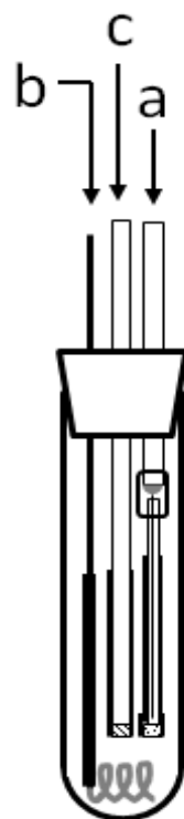
Fig. 2-5 Schematic illustration of the electrochemical cell. (a) Reference electrode, (b) counter electrode and (c) working electrode.
