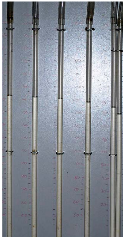
Fig. 3.22: End of the pump test for MS at 4 liters/min (15.3 cm)
