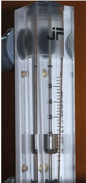
Fig. 3.19: Flowmeter at 20 liter/min
