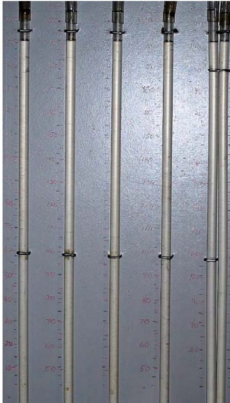
Fig. 3.21: Start of the pump test for MS at 4 liters/min (0.0 cm)
