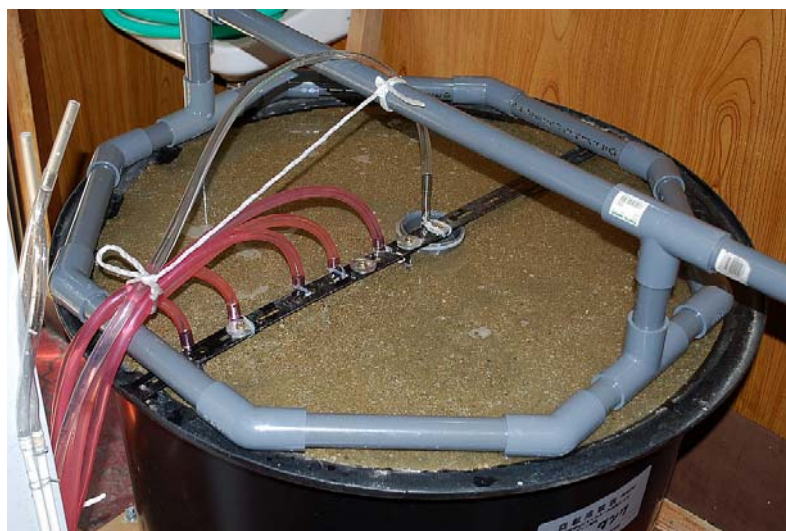
Fig. 3.18: 200 liter tank filled with saturated sediments
