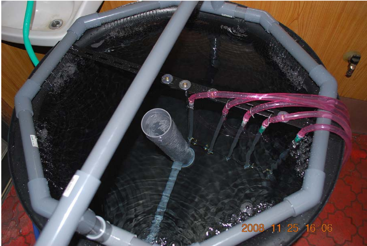
Fig. 3.8: Top view showing the center slotted pipe, plumbing, recharge ring, and water level tubes
