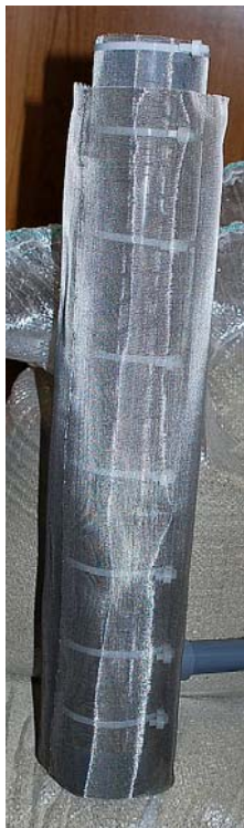
Fig. 3.13: Double layer screened center pipe
