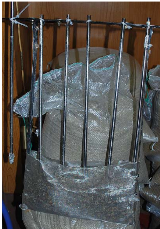
Fig. 3.14: Screened water level tubes with gravel packing
