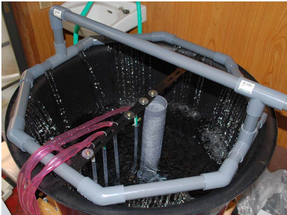
Fig. 3.10: Oblique view of the water level tubes, center slotted pipe, and recharge ring
