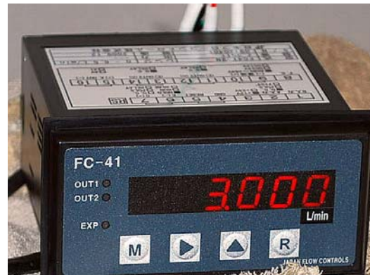
Fig. 3.20: Digital flowmeter at 3 liters/min
