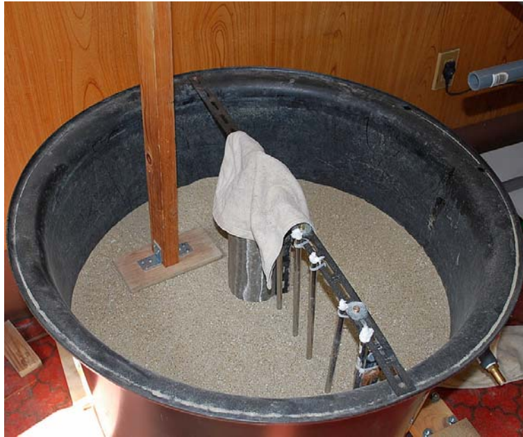
Fig. 3.17: Filling and tamping the tank with sediments
