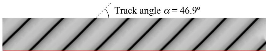
Fig. 3.3 The maximum pressure history on the wall in the case of steady mode.
