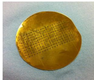
200 EDMed features on silicon wafer
