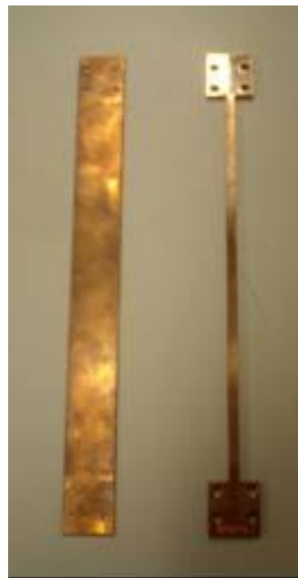
Figure 5.2. Healthy (Left) and Damaged (Right) Columns
