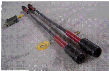
Figure 3 Smart cables with OFBG sensors Figure 4 Weigh-in-motion with OFBG sensors
