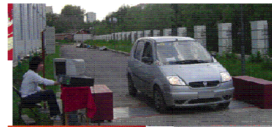
Figure 3 Smart cables with OFBG sensors Figure 4 Weigh-in-motion with OFBG sensors
