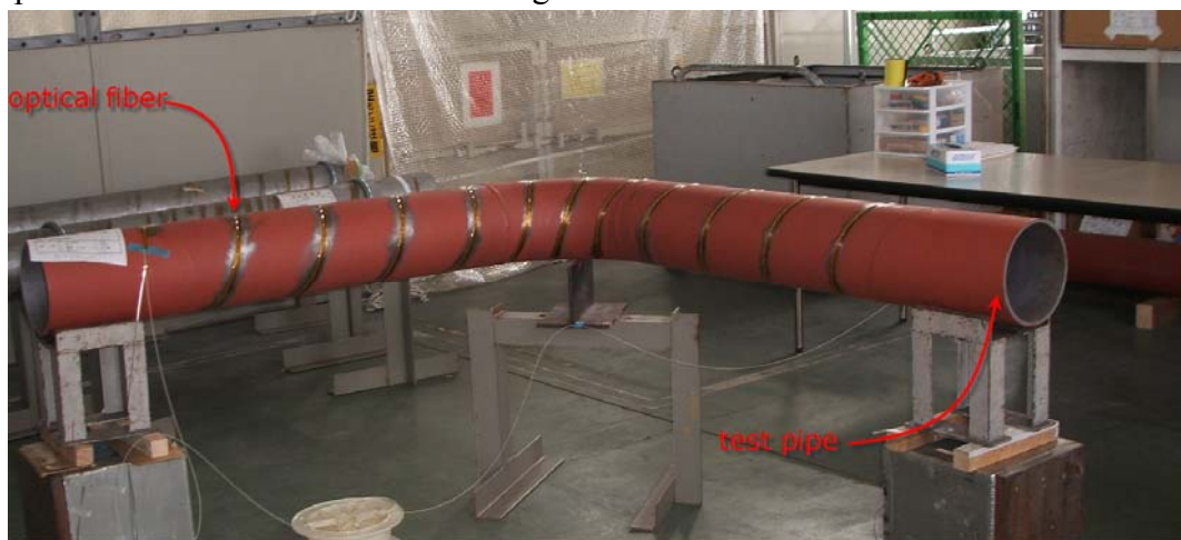
Figure 4: Specimen for thinning detection test.
