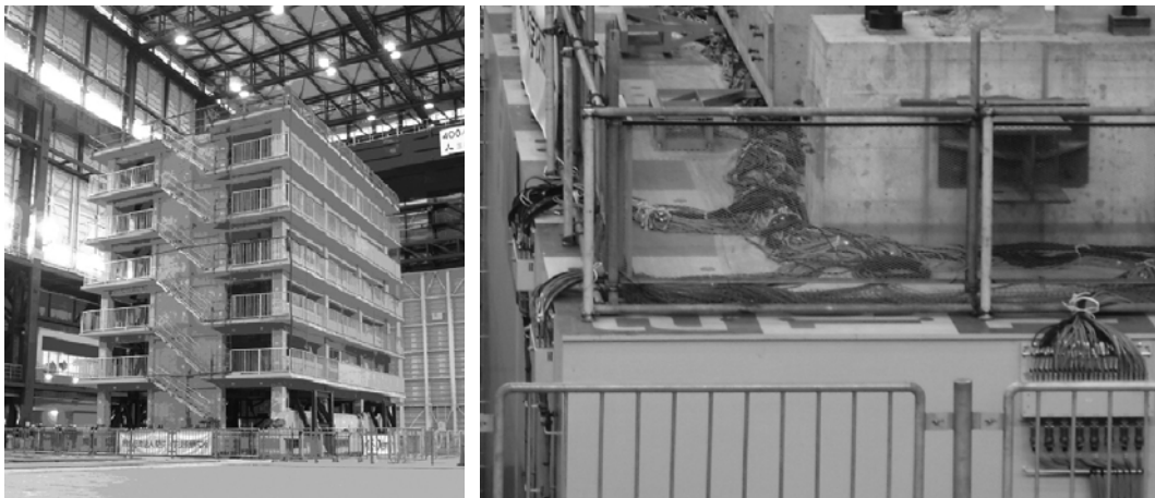
Figure 2: Many cables (A vibration destruction experiment at E-Defense)
